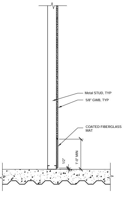
NOTE: BOTTOMS OF ALL PARTITITIONS TO CONTAIN ONE OR MULTIPLE LAYERS OF 5/8" COATED FIBERGLASS MAT PRODUCT BY NATIONAL GYPSUM COMPANY GOLD BOND BRAND EXP INTERIOR EXTREME AR GYPSUM PANEL. AT A MINUMUM STANDARD, DEPENDING ON THE APPROPRIATE WALL TYPE, CRITERIA, AND LOCATION.
